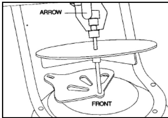
3. Install impeller on to pinion shaft by pushing down until you can install 1/8 x 1-1/4" cotter pin through the cross hole in the impeller and the pinion shaft. (**NOTE: Impeller fins must point away from the gearbox as shown.**)
