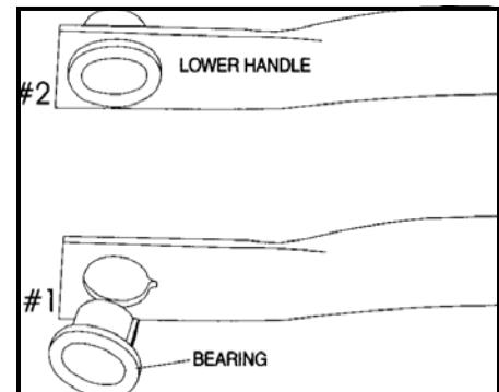
5. Insert nylon bearings into lower handles.
